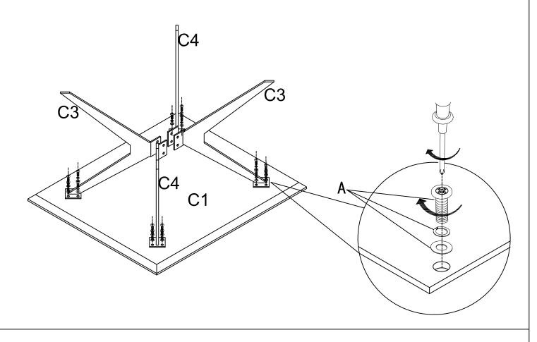
STEP 2:Use the Hex Key(C) to tighten the Legs(C3,C4) to the Leg Rail Panel(C2) with T Nut(B).
